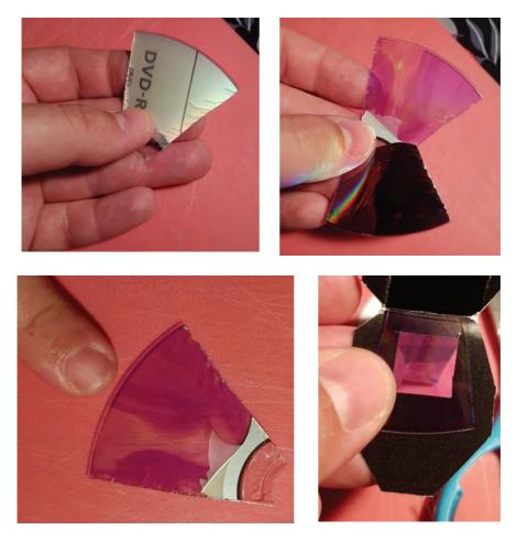
**Note:** It's important the DVD is cut and placed the right way. The curvy part of the DVD should face towards the bottom of the 'window' slit (see below). If the DVD faces the wrong way the colour lines will not show up in the right place.
