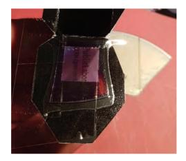
7. Secure the body, slit end, and window end of the spectrometer.
