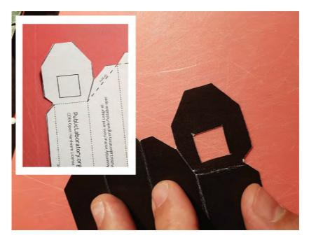
4. Cut a slit - make sure it is nice and thin. You might need to make the slit bigger, but for now, keep it small. It is easier to make a small slit bigger, but very hard to make a big slit smaller.
